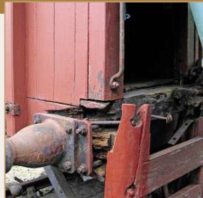
The bufferbeam of NER plough No 18 before rebuilding.
